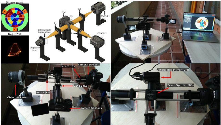
**Fig. 7.** Proof-of-concept optical system. We build our optical architecture with two CANON cameras, one objective CANON lens, three lenses, one beam splitter, and one deformable mirror. For more details please see the supplementary video.
